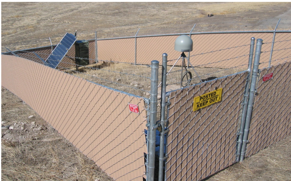
A PBO GPS station that was vandalized and subsequently had a security fence installed. Multipath values increased by 50% after the fence was installed.
