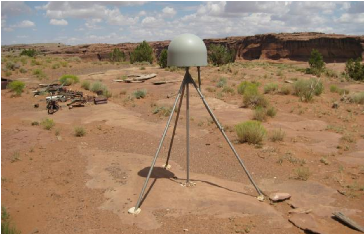
A GPS monument (SDBM) installed in highly competent sandstone
